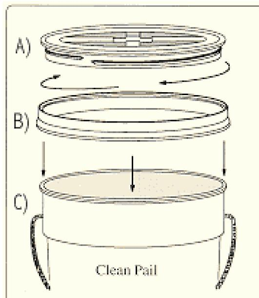
Figure 1: The Gamma Seal lid (A), screws into the adapter (B), which is fitted onto the lip of an ordinary plastic bucket (C). (The Bread Beckers 2002)
