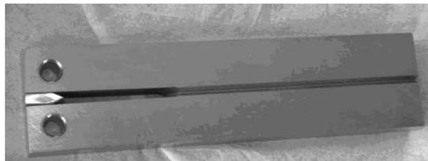
**Fig. 1** Pictorial view of the DCB specimen
