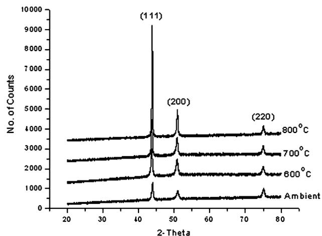
Fig. 7 XRD profile versus temperature
