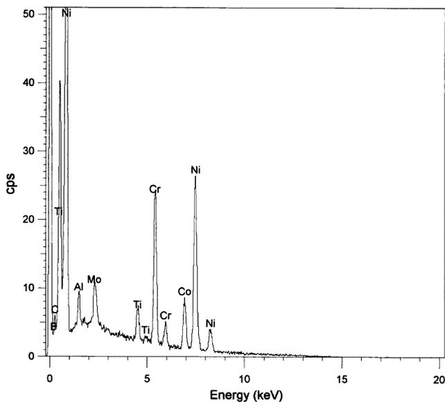
Fig. 6 EDS spectrum for specimen tested at 800 °C
