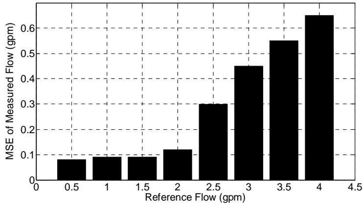
Fig. 3.8. Mean square error of measured flow
