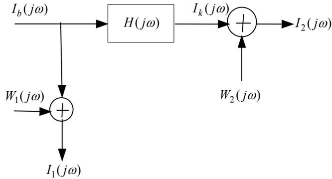
Fig. 2.3. Transfer function estimation with added white noise.
