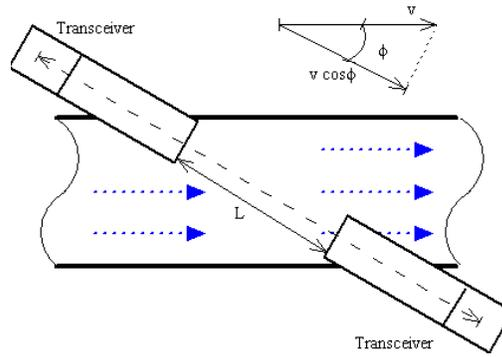
Fig. 4.2. A schematic of the transit-time ultrasonic flowmeter.
