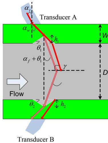
Fig. 4.8. Schematic diagram of the Doppler ultrasonic transducer.
