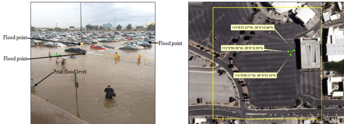
Figure 10. Imagery used for model calibration showing the location of some of the known flood points and the peak depth location at the inlet where watermark was still intact after flooding (on the left) verified through a field visit, and the exact geographic location of the points recorded via field visit with a GPS (on the right). Courtesy of Rebel Yell, University of Nevada Las Vegas.
