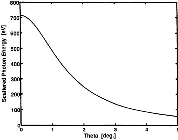
FIGURE 2. The scattered photon energy as a function of the angle of declination from the initial electron beam velocity. A Gaussian profile, focused, 2-J pulsed, CO<sub>2</sub> laser beam collides head-on with a Gaussian profile, 20-MeV, 3-nC, pulsed electron beam. Both beams have a 10-mm beam waist. The electron and photon pulse durations are, respectively, 500 ps and 5 ns.
