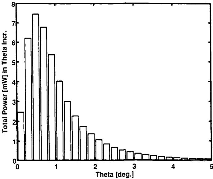
FIGURE 3. The total power in angular bins of  $\Delta\theta = 0.2^\circ$  for the head-on collision between the CO<sub>2</sub> laser beam and the electron beam of figure 2.
