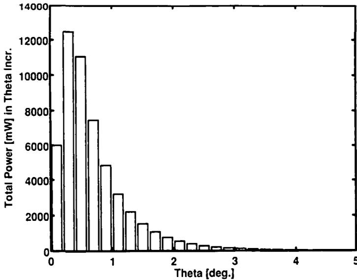
FIGURE 5. The total power in angular bins of  $\Delta\theta = 0.2^\circ$  for the head-on collision between the ruby laser beam and the electron beam of figure 4. Sensitive detectors are capable of measuring powers of this magnitude.
