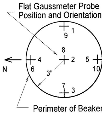
FIG. 6. Sketch of the probe positions inside the region of a beaker in which experiments are conducted. Based on theory and calibration measurements, the exact placement of the beaker at the coil center is not crucial. Allowances have been made in the coil design for the volume of field uniformity to be much larger than the experimental volume actually used.
