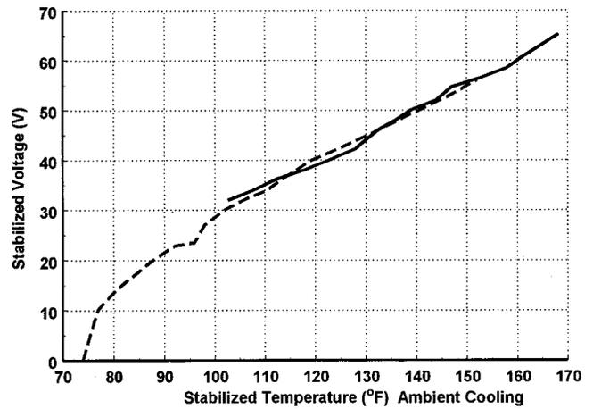
FIG. 4. Steady state temperature of the coil was monitored relative to the voltage applied to the Helmholtz coil by an autotransformer directly connected to a utility outlet. The voltage supplied to the coil was monitored by a Tektronix digital multimeter. Two sets of data taken at different times have been plotted. The ambient Helmholtz coil resistance in parallel configuration is 2.5  $\Omega$ .
