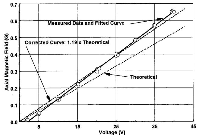
FIG. 5. Theoretical, measured, and corrected axial magnetic field plotted against the voltage measured across a known resistor connected in series with the coil. Note that the experimental data fits along a linear curve that does not pass through the origin. Four data points were taken at 5 V increments. At the 2 V level note that the recorded data begins to deviate from the fitted curve. The position of the probe was fixed on the *z* axis about 1/32 in above the geometrical center of the coil.
