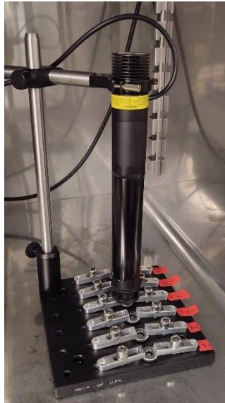
Figure 2. Optical setup with coupons secured in wells for UVC testing, located in the incubator.
