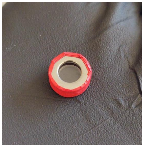
Figure 3. An ETT coupon pressed between two of the plating washers to measure UVC ETT transmission.
