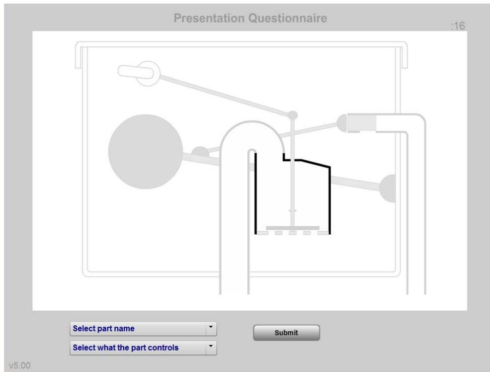
Figure 4. Screen shot of a Parts-Recall question for "siphon bell".
