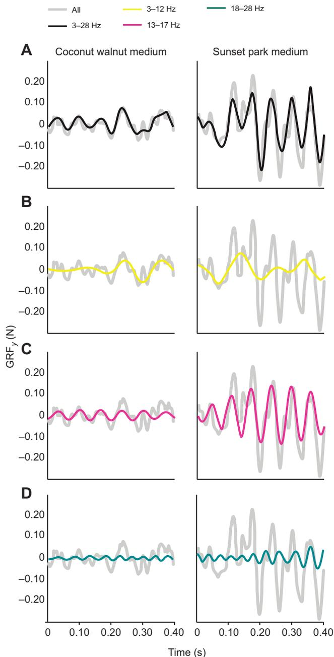
**Fig. 2.** Traces of fore–aft ground reaction force ( $GRF_y$ ) from the entry tube, together with Fourier reconstructions using terms in the frequency ranges specified by color. (A) 3–28 Hz, (B) 3–12 Hz, (C) 13–17 Hz, (D) 18–28 Hz. The signals are zeroed by subtracting the offset as the first step in Fourier analysis.
