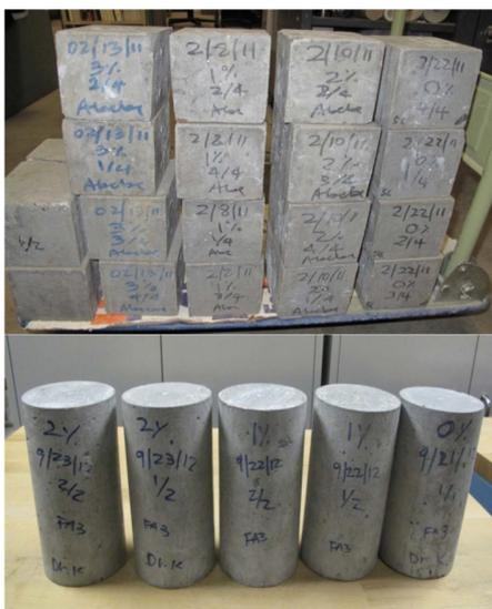
Fig. 1. Prepared beam and cylindrical samples.
