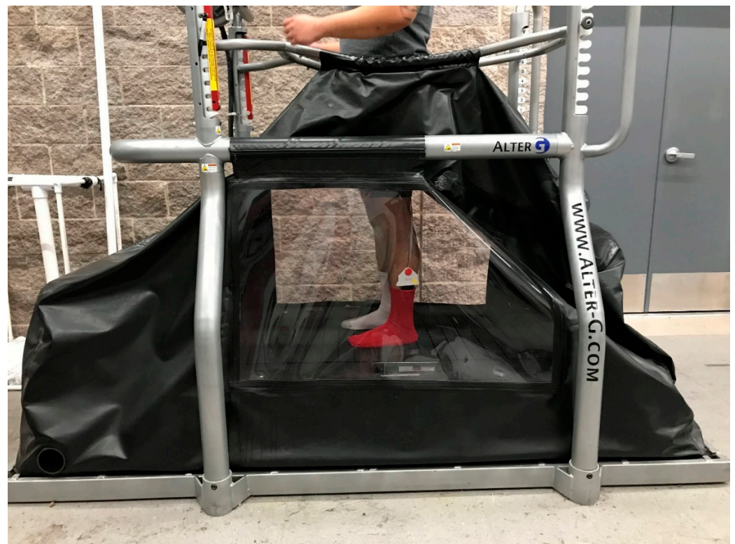
Figure 1. Subject using AlterG ® Treadmill with Medilogic ® Pressure-Measuring Insoles.
