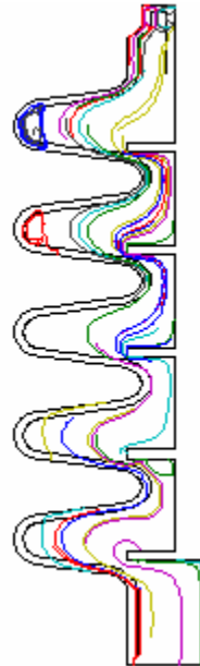
Figure 44. Flow line plot for case 12 ( v_5=0.08 ) of parameter study 1
