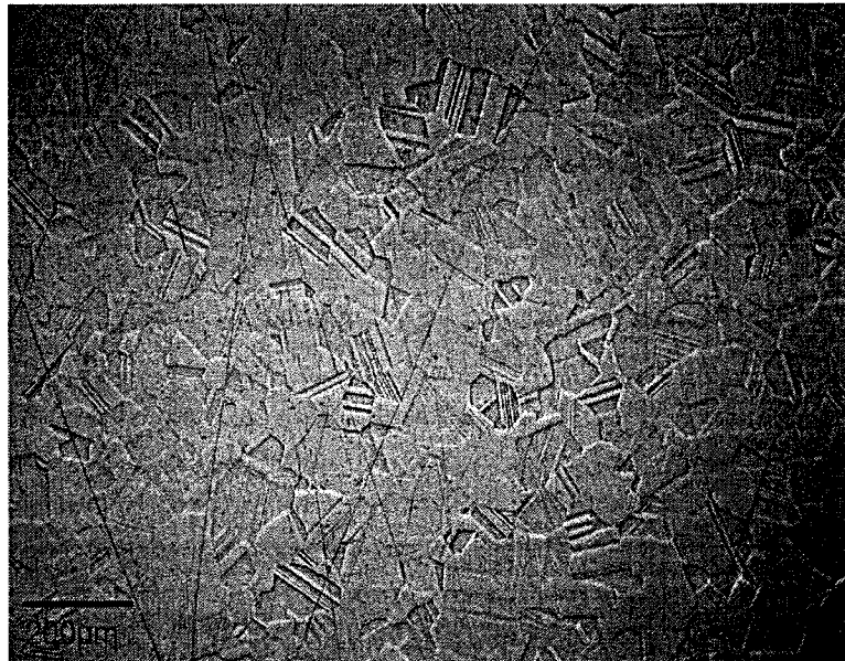
Figure 4-1 Optical Micrograph, Etched (Glyceregia), 50X
