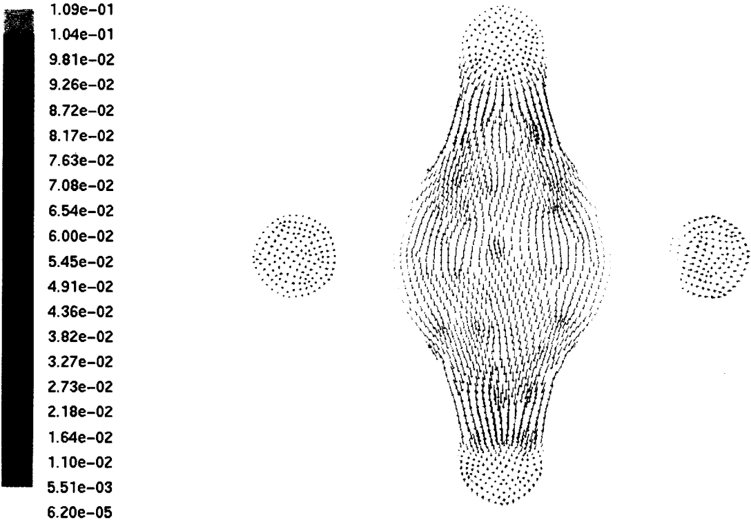
Figure 4.7 Velocity vectors (m/s) on a plane taken perpendicular to the HP-RACE Target's axis through a water channel with an input volumetric flow rate of 0.535 L/min.
