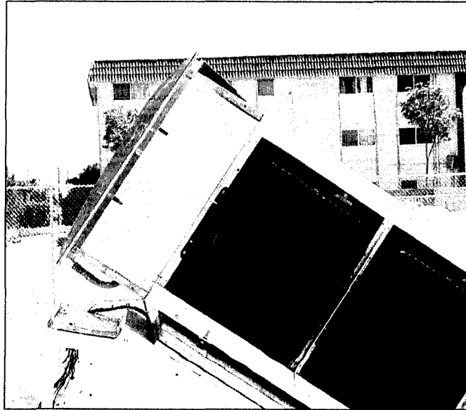
Figure 15 BCS target with air dams mounted on the heat rejection system
