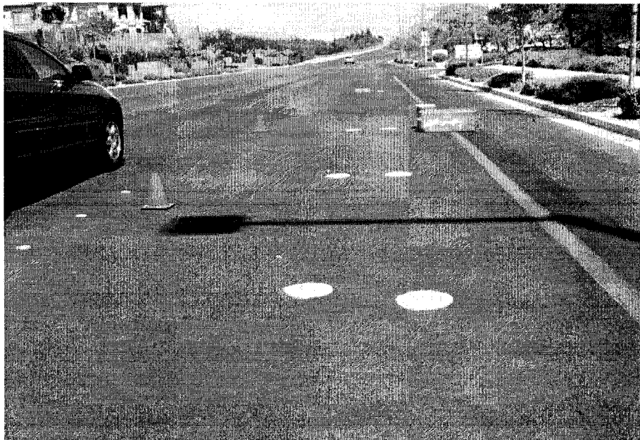
Figure 3.3 Sand Patch Experiment (Crestdale & Covington Cross)
