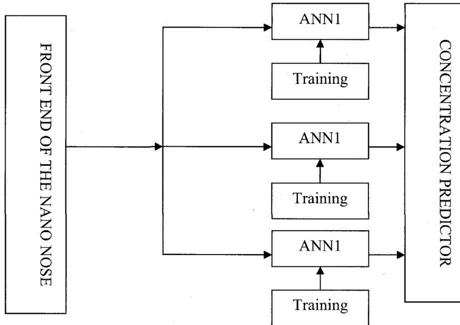
Figure.3.1 Block diagram of the mixed gas detector
