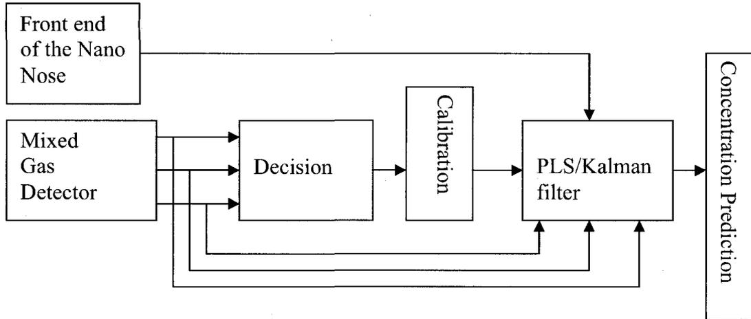
Figure 4.1 the block diagram of the gas concentration predictor
