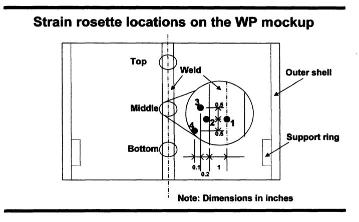
Figure 6.2. SNF Canister Mock-up and Strain Rosette Locations
