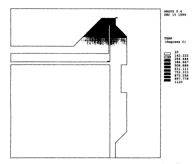
Figure 5.1. Temperature Distribution in the 2-D Axisymmetric FEM (Time: 35 seconds)
