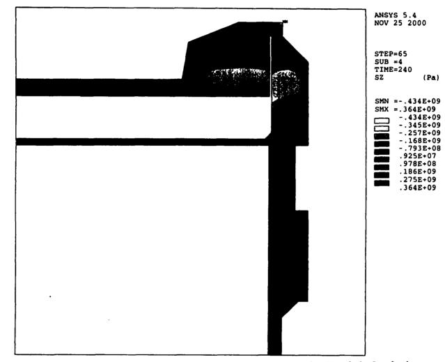
Figure 7.19. Hoop Stress Distribution for the Successive Heuristic Quadratic Approximation Solution (Time: 240 seconds)
