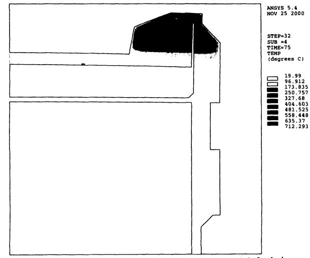
Figure 7.12. Temperature Distribution for the Successive Heuristic Quadratic Approximation Solution (Time: 75 seconds)
