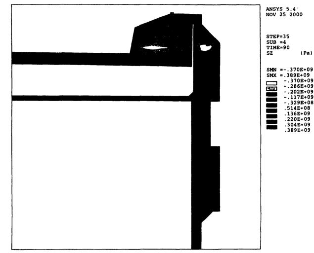
Figure 7.15. Hoop Stress Distribution for the Successive Heuristic Quadratic Approximation Solution (Time: 90 seconds)
