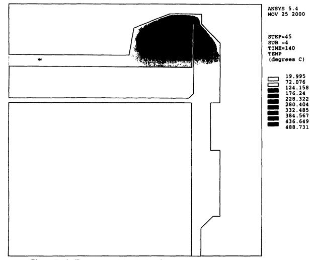
Figure 7.16. Temperature Distribution for the Successive Heuristic Quadratic Approximation Solution (Time: 140 seconds)
