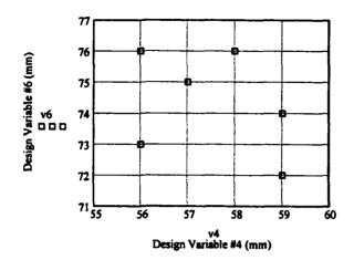
The design variable plot given above indicates that the minimum stress value (-158,272,820 Pa corresponding to V4 = 57 mm, V6 = 75 mm), is surrounded by higher stress values. Therefore, the minimum stress value (-158,272,820 Pa) is an optimum solution.
