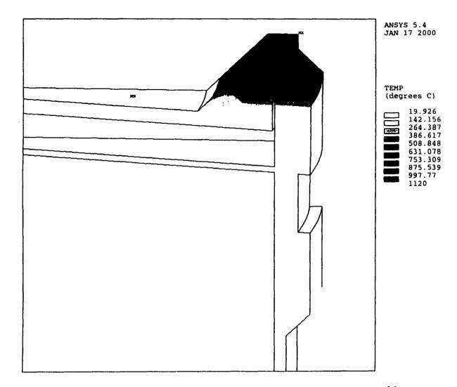
Figure 4.3. Temperature Distribution in the SNF Canister (Time: 35 seconds)
