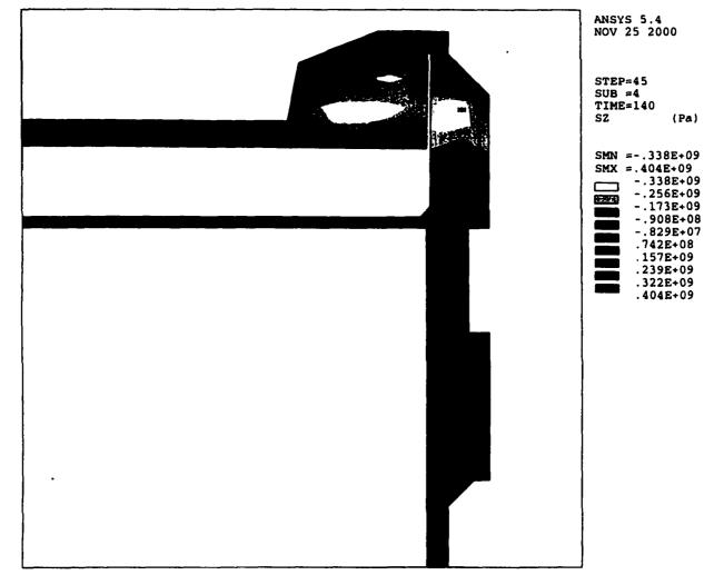
Figure 7.17. Hoop Stress Distribution for the Successive Heuristic Quadratic Approximation Solution (Time: 140 seconds)
