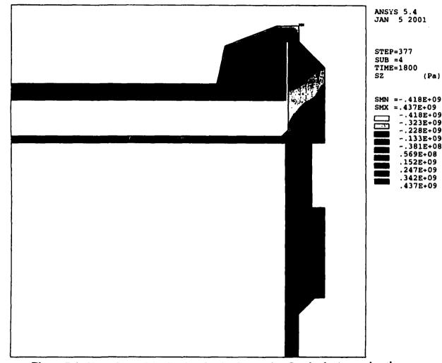
Figure 7.6. Hoop Stress Distribution for the Successive Quadratic Approximation Solution (Time: 1800 seconds)
