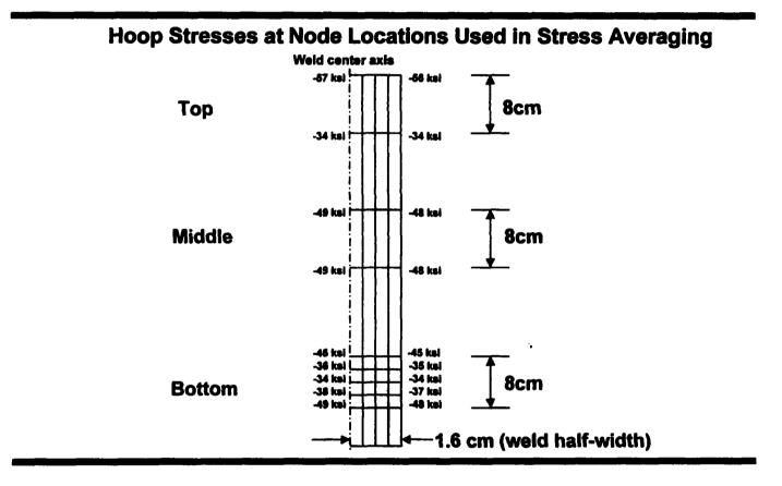
Figure 6.6. SNF Canister Mock-up Hoop Stresses at Nodes Used in Stress Averaging
