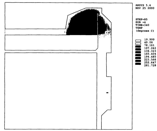
Figure 7.20. Temperature Distribution for the Successive Heuristic Quadratic Approximation Solution (Time: 340 seconds)
