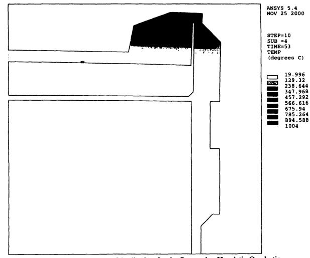
Figure 7.10. Temperature Distribution for the Successive Heuristic Quadratic Approximation Solution (Time: 53 seconds)
