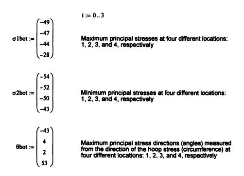
Hoop stresses at the bottom locations in the canister mock-up:
