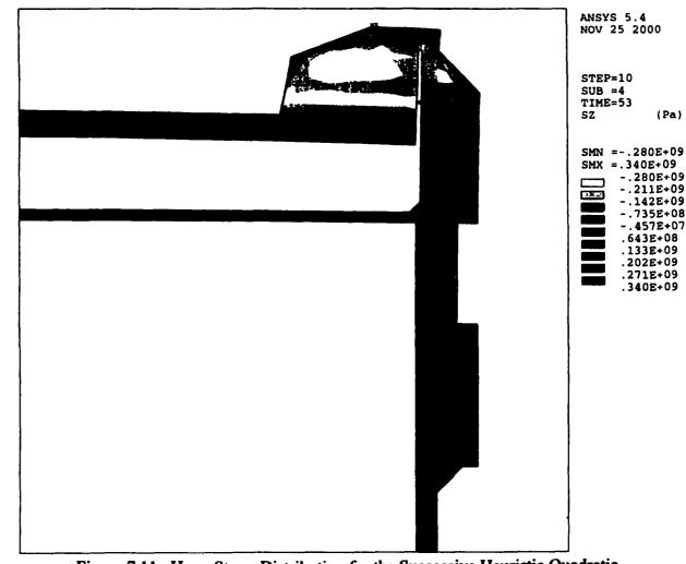
Figure 7.11. Hoop Stress Distribution for the Successive Heuristic Quadratic Approximation Solution (Time: 53 seconds)
