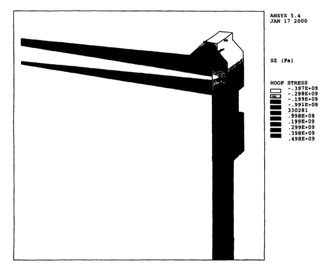
Figure 4.4. Residual Hoop Stress Distribution in the SNF Canister
