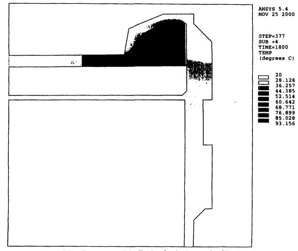
Figure 7.22. Temperature Distribution for the Successive Heuristic Quadratic Approximation Solution (Time: 1800 seconds)
