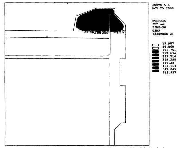
Figure 7.14. Temperature Distribution for the Successive Heuristic Quadratic Approximation Solution (Time: 90 seconds)
