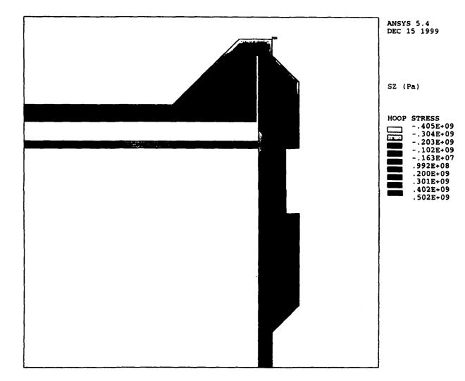
Figure 5.2. Residual Hoop Stress Distribution in the 2-D Axisymmetric FEM
