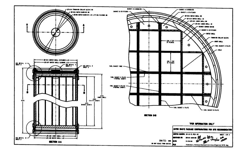
Figure 3.1. Spent Nuclear Fuel Canister Design Sketch (General View)
