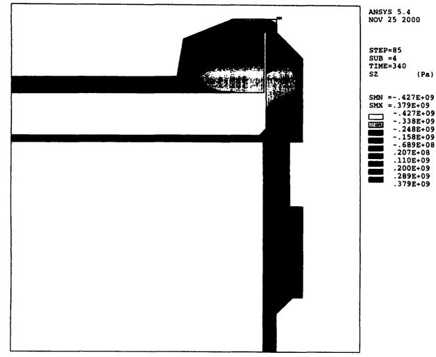
Figure 7.21. Hoop Stress Distribution for the Successive Heuristic Quadratic Approximation Solution (Time: 340 seconds)
