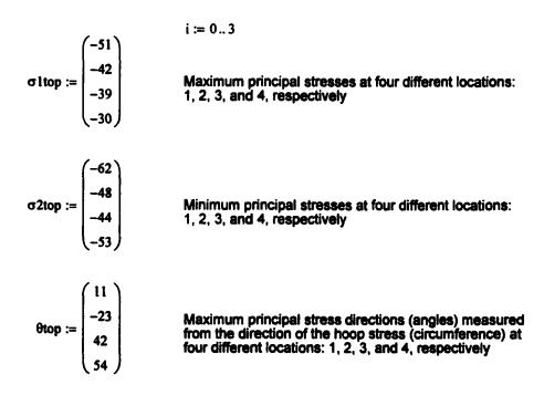
The magnitudes of the hoop stresses are obtained using the following relation from the Mohr's circle for biaxial stress state:
