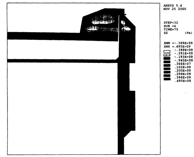
Figure 7.13. Hoop Stress Distribution for the Successive Heuristic Quadratic Approximation Solution (Time: 75 seconds)
