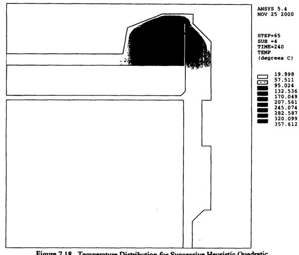
Figure 7.18. Temperature Distribution for Successive Heuristic Quadratic Approximation Solution (Time: 240 seconds)
