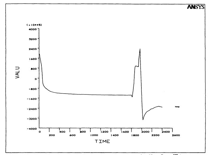
Figure 6.5. SNF Canister Mock-up Ring Area Outer Shell Surface Hoop Stress History (Hoop stress in Pa, Time in seconds)
