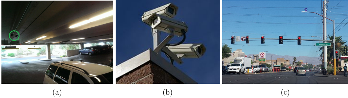
Figure 1.1: Examples of real surveillance cameras. a A license plate recognition camera (green circle) pointing up the ramp to view vehicles entering the SEB garage at UNLV. b Surveillance cameras high atop the the corner of a building [1]. c Intersection monitoring camera (blue circle) on top a light post over a Las Vegas road.
