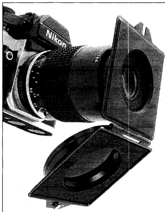
Figure 3-4. UV-Nikkor lens and Nikon UV-transmittive filter. Copyright by Stephen Gandy, www.CameraQuest.com . All Rights Reserved.
