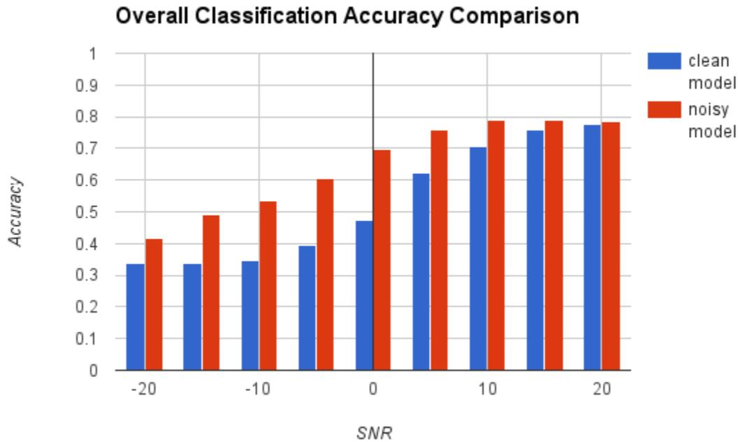
Figure 8: Comparison of the average accuracy of both classifier models across all noise types versus SNR
