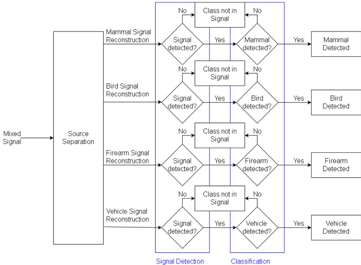
Figure 1: System diagram
