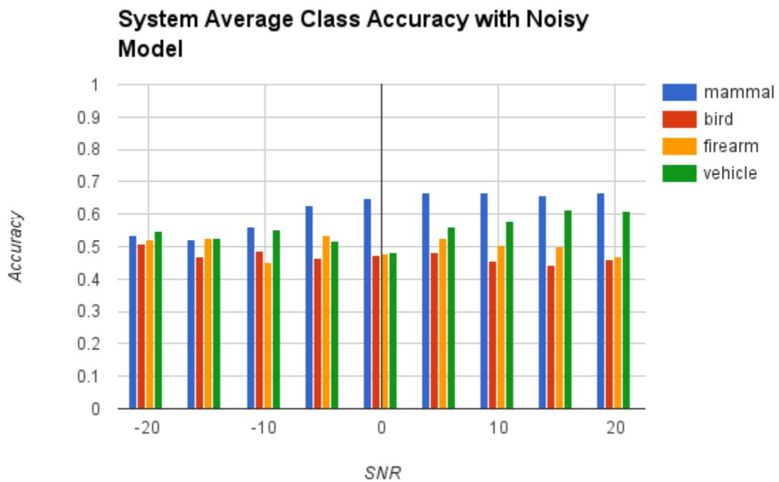
Figure 17: System accuracy for each class versus SNR, while using the noisy classifier
