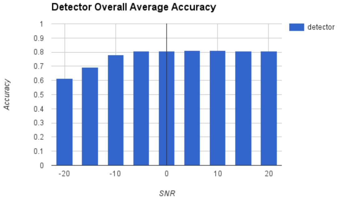
Figure 6: Average detector performance across all noise types versus SNR
