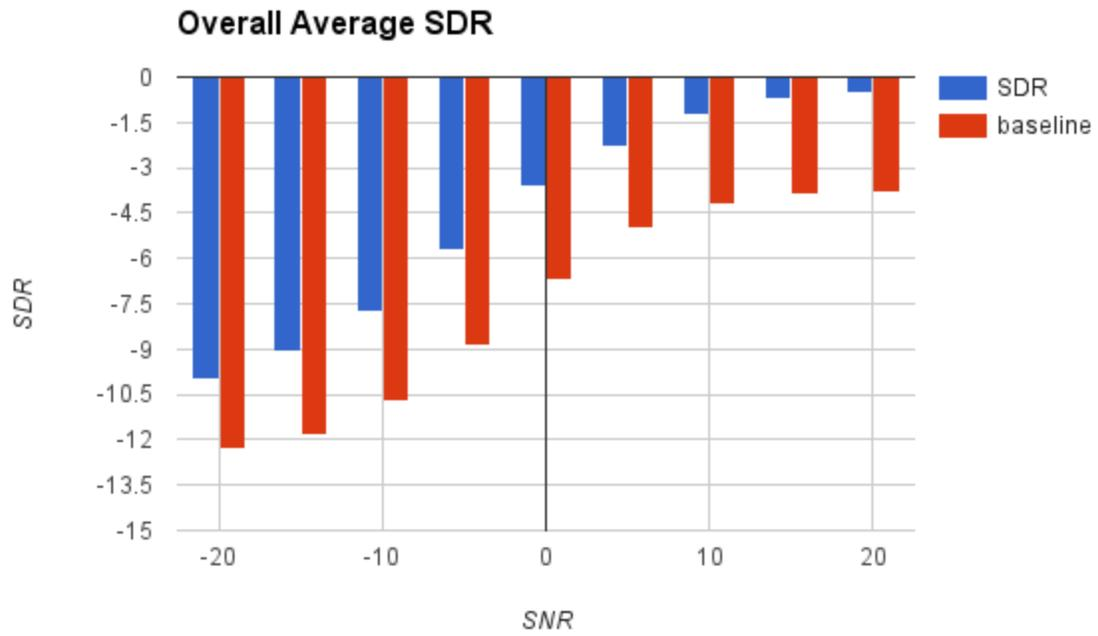
Figure 3: Average SDR across all noise types versus SNR
