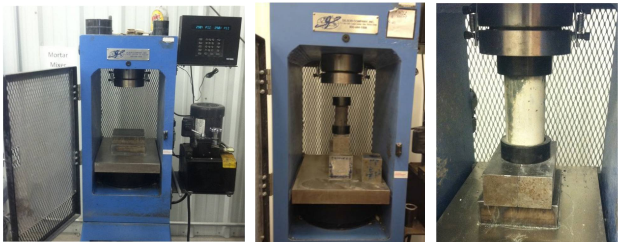
Figure 3.10 Compressive strength test setup
