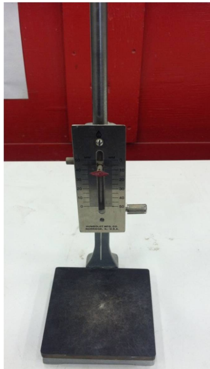
Figure 3.8 Setting time test device
