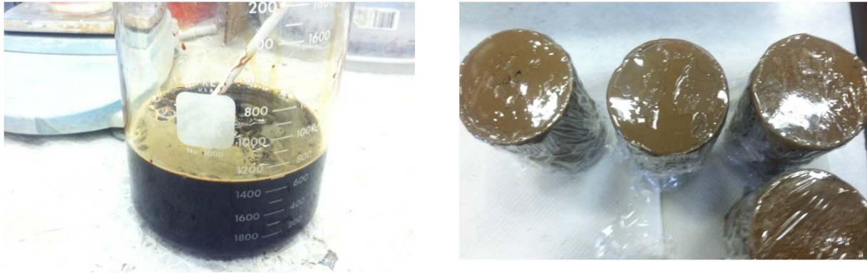
Figure 4.5 Use of lignosulfonic acid sodium salt, (a) combination with sodium hydroxide, (b) produced alkali-activated paste samples
