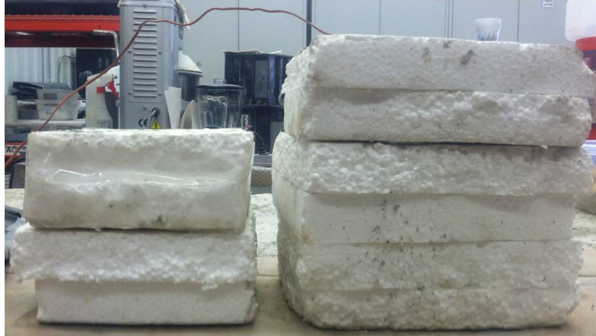
Figure 3.9 The designed boxes for measurement of heat of hydration
