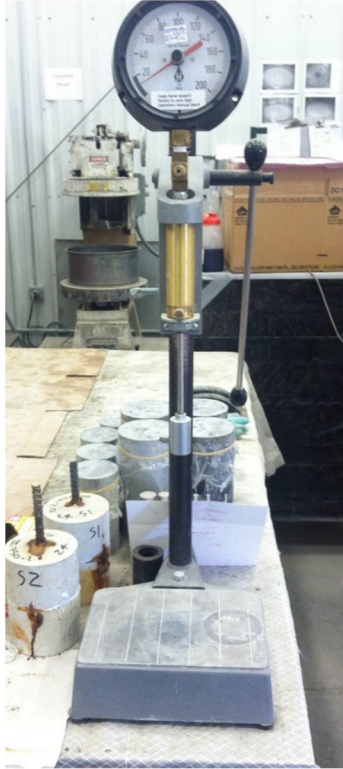
Figure 3.19 Setting time test device for concrete
