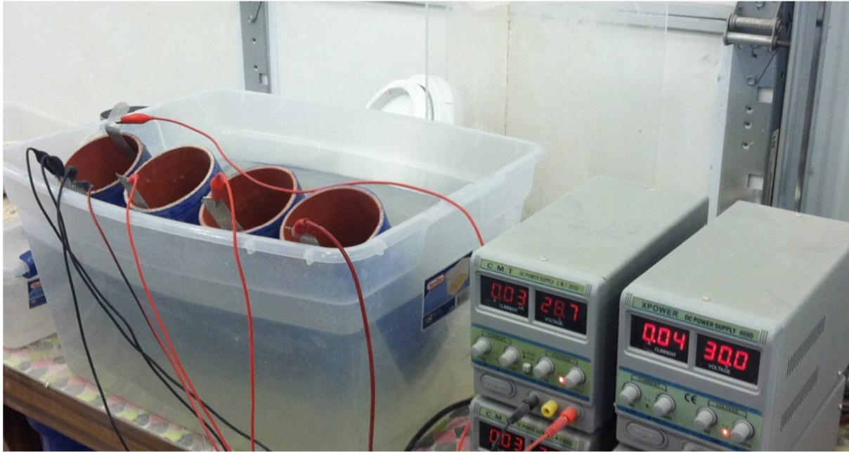
Figure 3.17 RMT test setup
