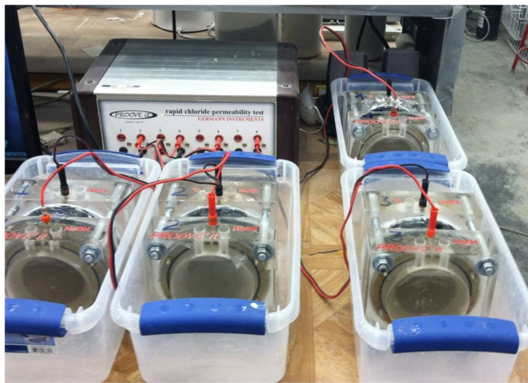
Figure 3.16 RCPT test cell and device
