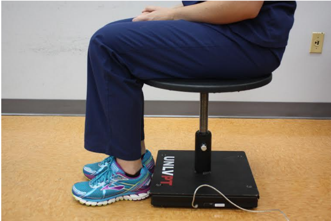
Figure 1. Force Plate Instrumented Stool
