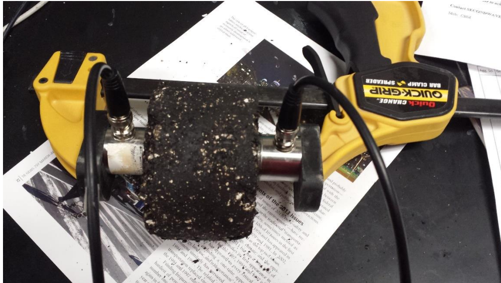
Figure 48. Sample fixed between two transducers
