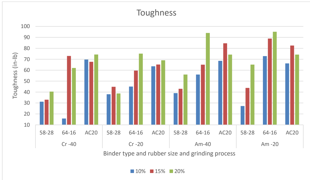
Figure 52. Toughness for binders mixed with CRM
