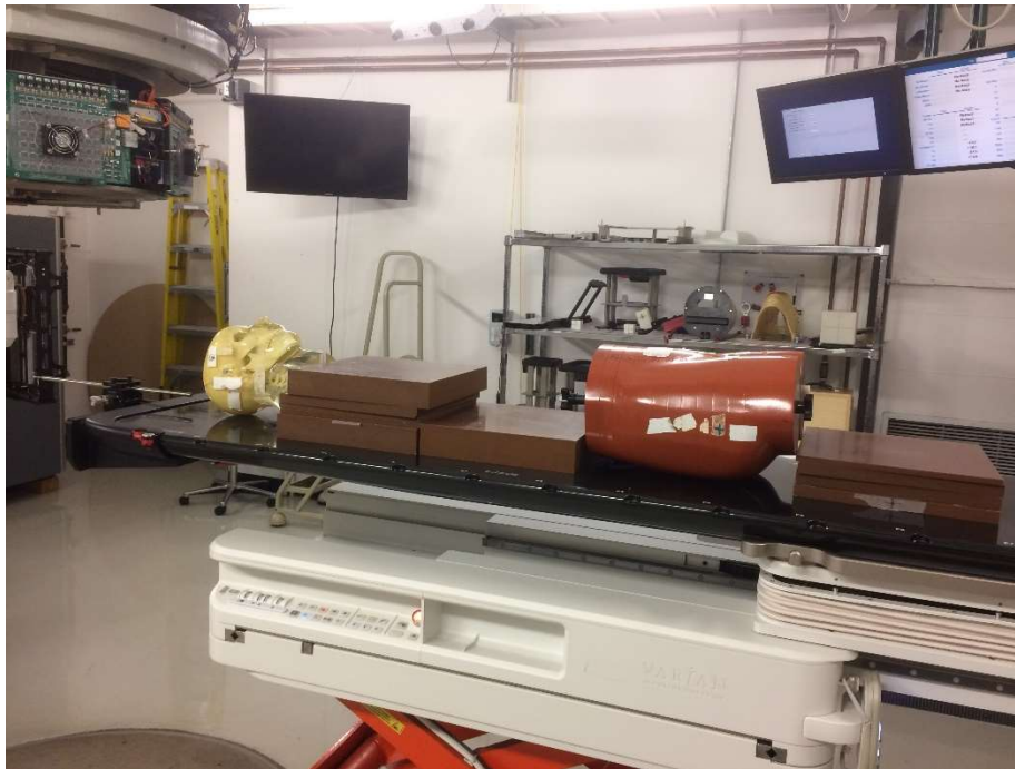
Figure 12: The weight-loaded couch to mimic the clinical situation
