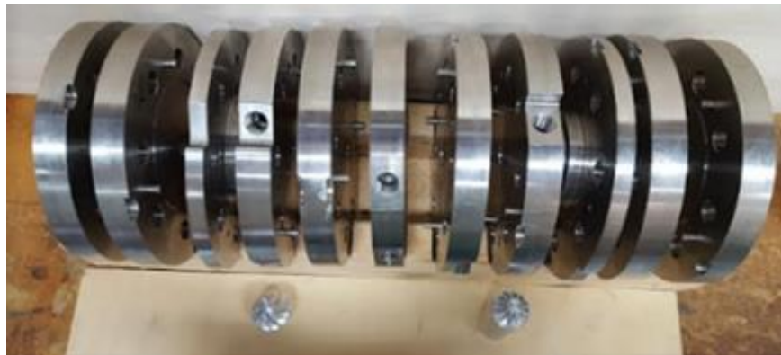
Figure 22. Turbomachinery Vane Plate Assembly
