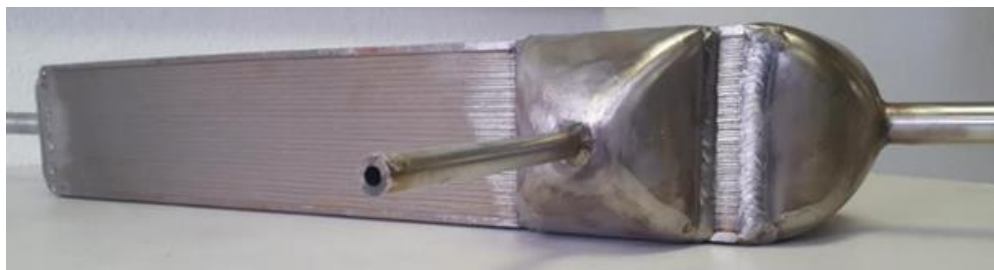
Figure 15. Xi'an Jiaotong University Printed Circuit Mini-Channel Heat Exchanger
