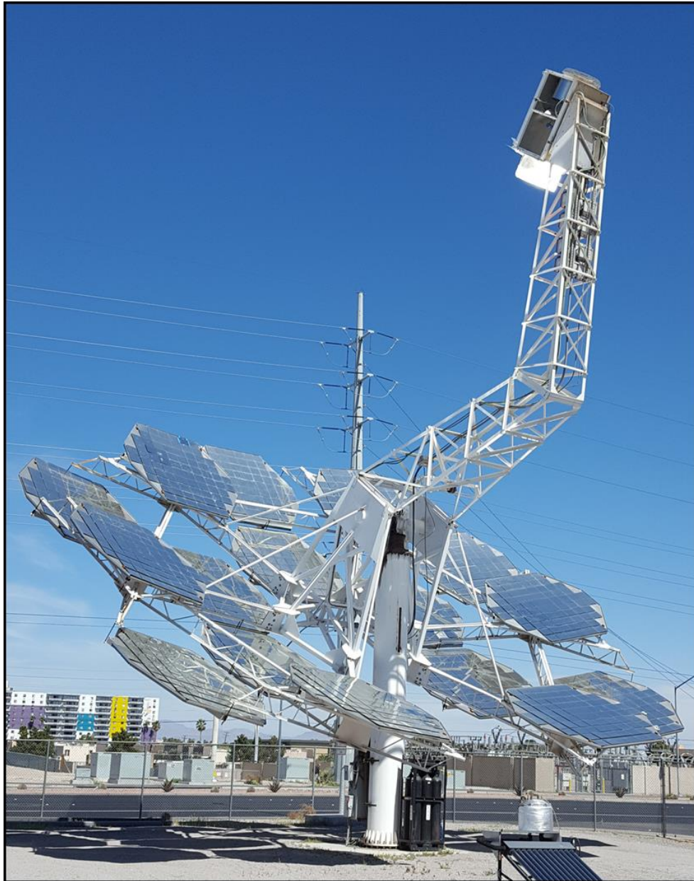
Figure 2. SAIC Dish On-Sun Testing
