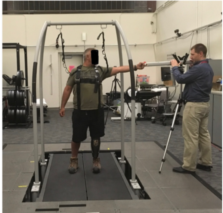
Figure 1: Original starting position in the overhead harness secured to the Bertec force plate.
