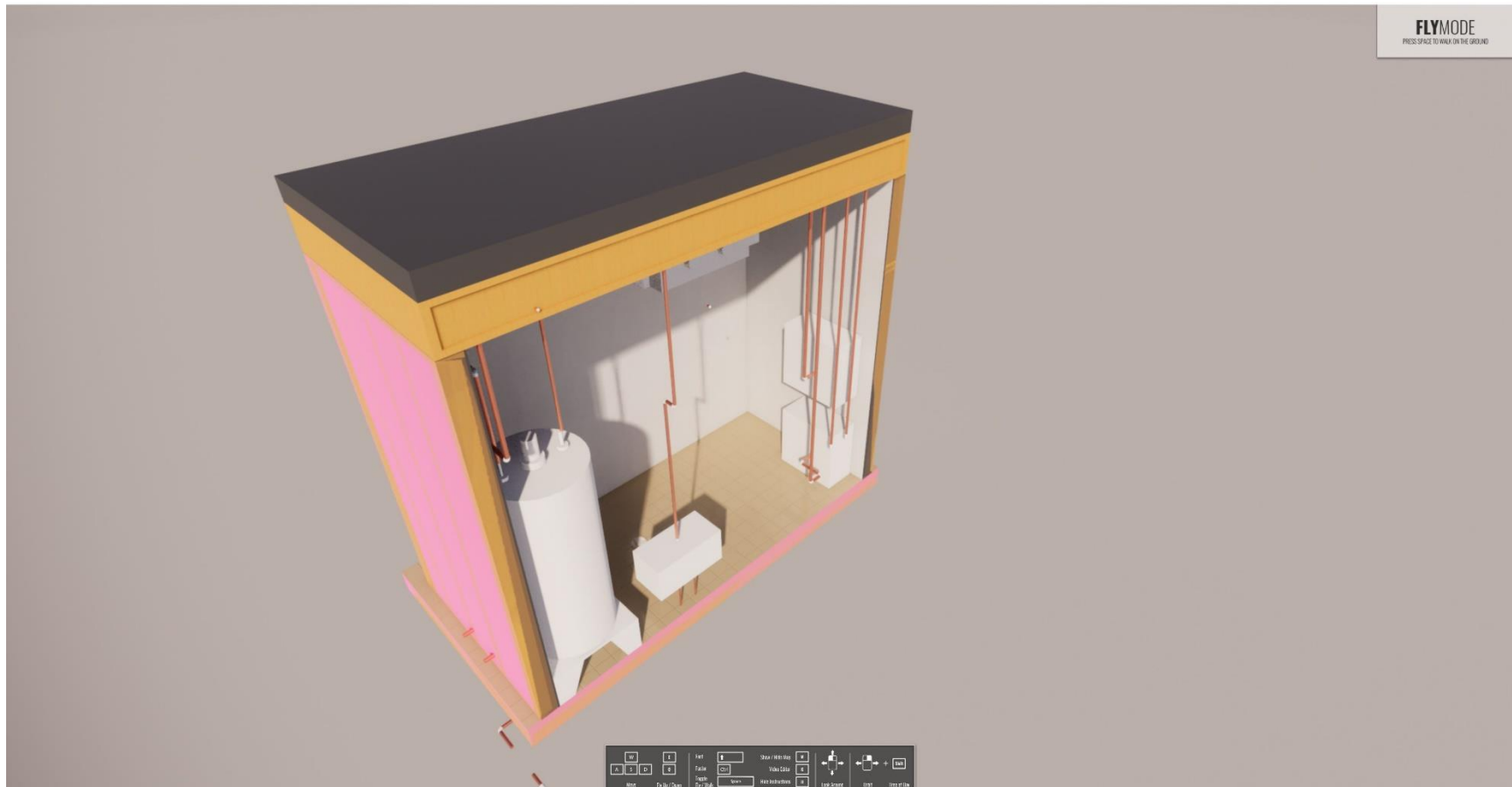
Module 1: Mechanical Room Module
