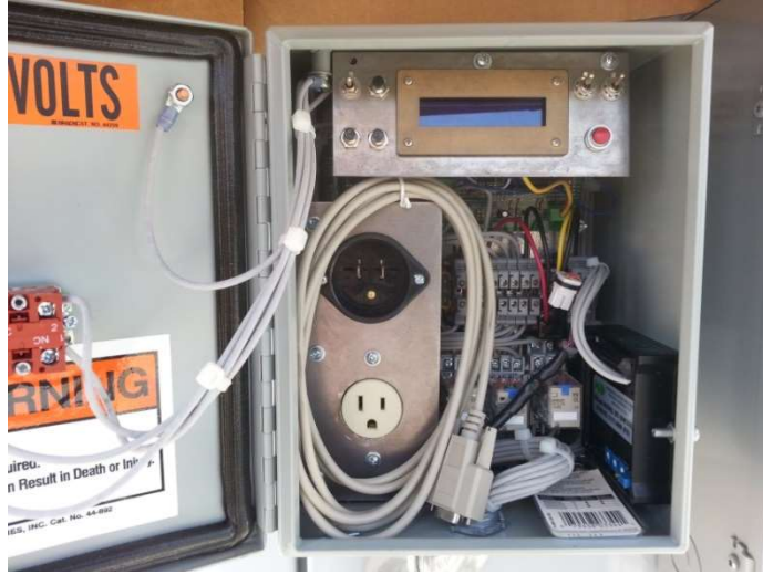
Figure 2.6 Frequency and Voltage Disturbances Controller.
