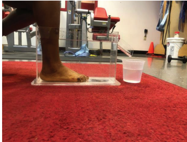
Figure 1. Foot Lucite Volumeter used for measuring foot volume changes
