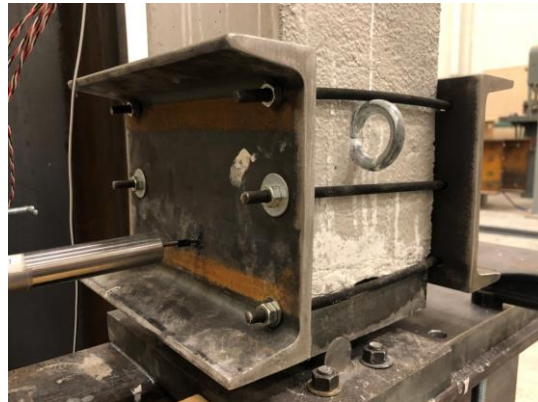
Figure 3.15 Confinement provided at column ends.
