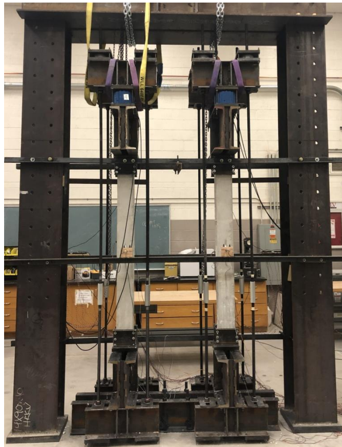
Figure 3.17 Two specimens installed prior to sustained eccentric loading test.
