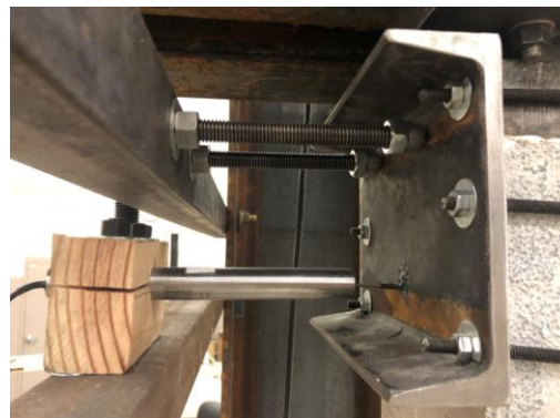
Figure 3.16 Lateral support at column upper end.
