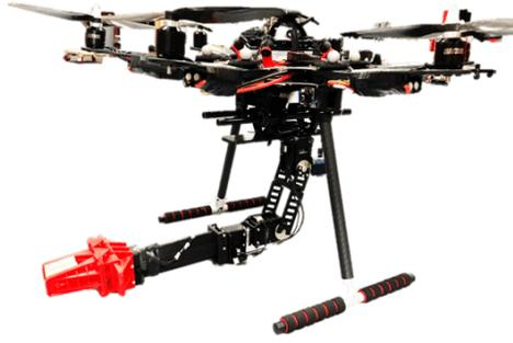
Figure 4.19: Close-up of Aerial Manipulator: a single arm and gripper is attached under drone's belly; a camera is attached close to the landing gear
