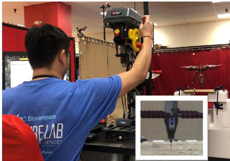
Figure 3.19: Aerial manipulation with a customized haptic drill press. Operator feels reaction forces on the manipulator (inset); Inset shows a rotary drill manipulator drill pressing on a plywood board
