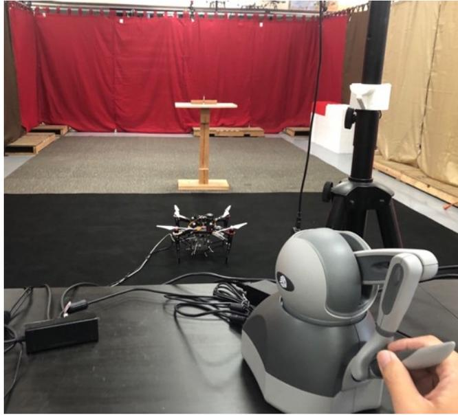
Figure 3.14: MM-UAV and spring test bench in the motion capture arena being controlled by the Touch haptic device
