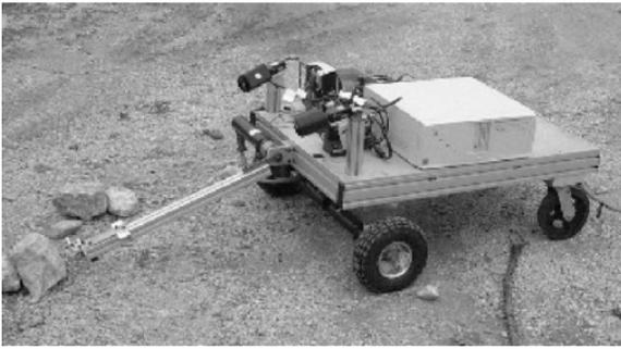
(a) NASA Rover Prototype [1]
