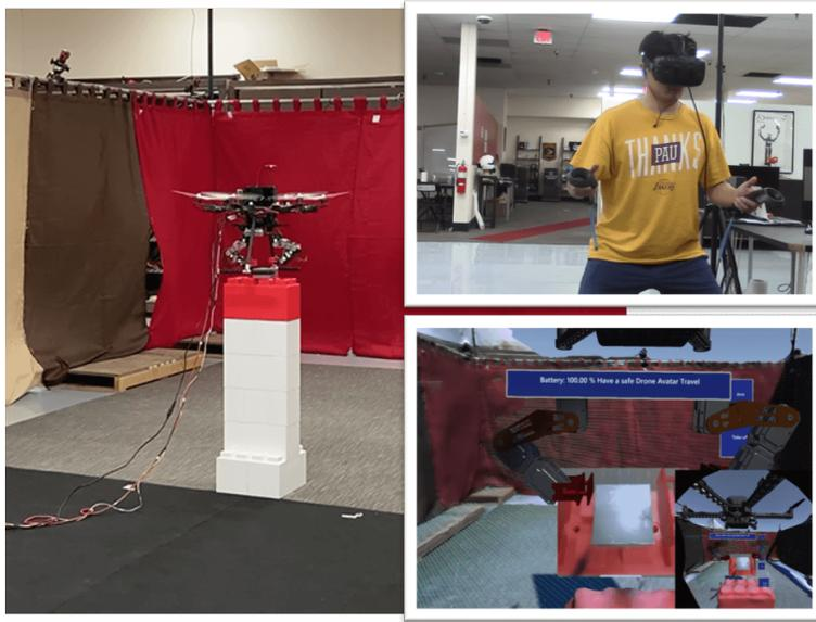
Figure 4.2: Human-embodied drone performing tasks in real world (left), operator in VR station (top right), View to the operator thorough VR headset (bottom right).
