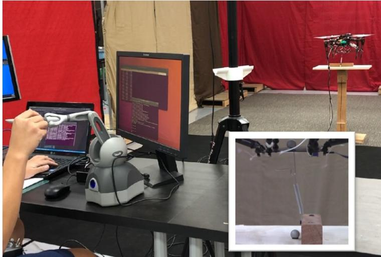
Figure 3.8: Aerial manipulation with a haptics device. Operator feels reaction forces on the manipulator (inset); Inset shows manipulator grabbing a spring
