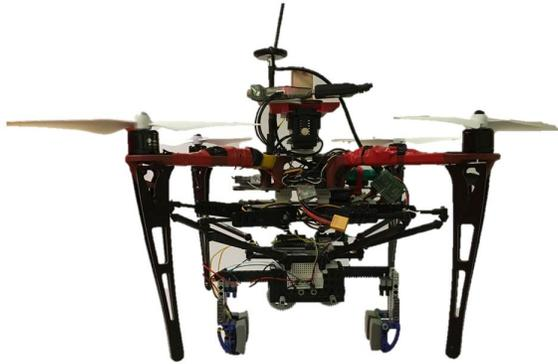
Figure 3.5: Lab automation drone prototype
