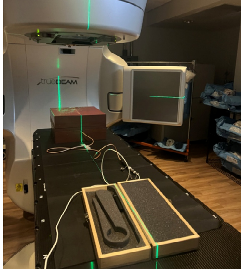
Figure 38. Solid water-based output & energy check setup for photon. SSD 100 cm, 100 MU, depth of 10 cm for 6x, 6xFFF, 10x, 10xFFF, 15x measurements.
