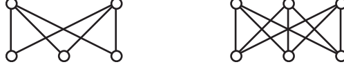
Figure 2.4: Two complete bipartite graphs K(2,3) is on the left and K(3,3) is on the right [20].
