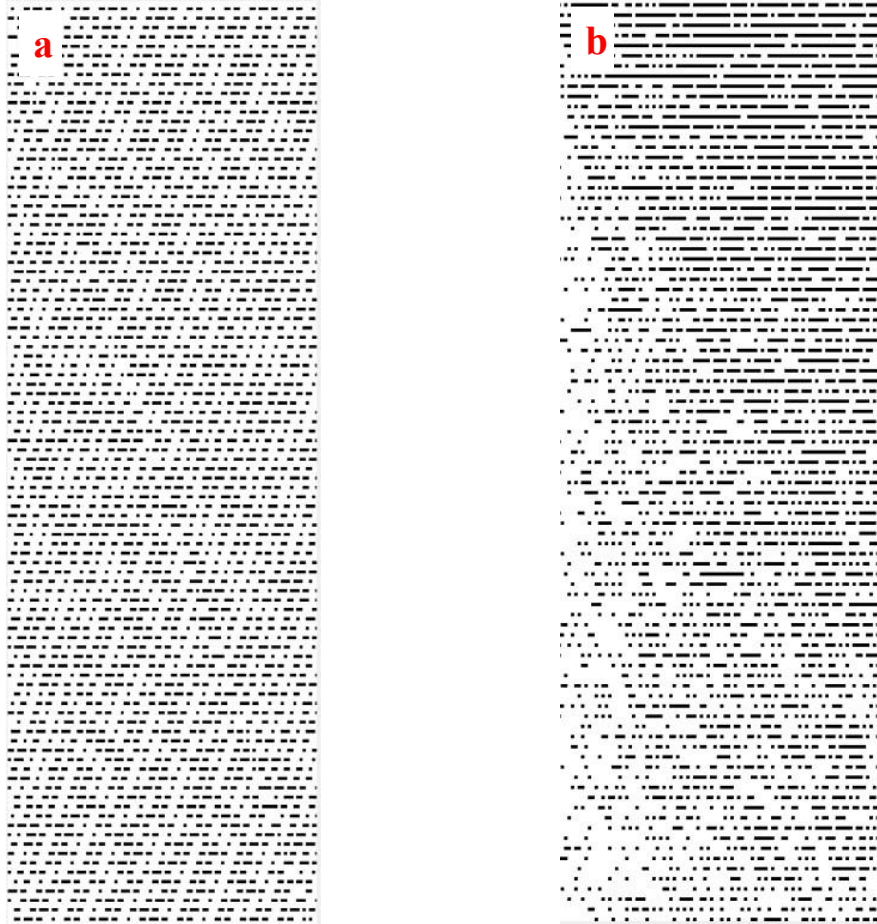
Fig. 5.3-1 (a) simulated quasi-random structures with low discrepancy value (more uniform); b) simulated pseudo-random structures with high discrepancy value (more random).
