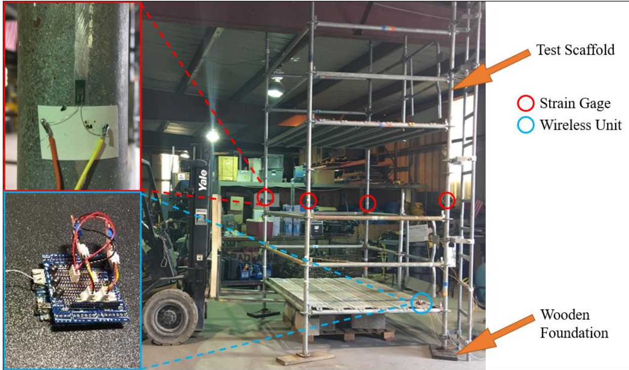
Figure 13. Test Scaffold with Strain Sensors Installed
