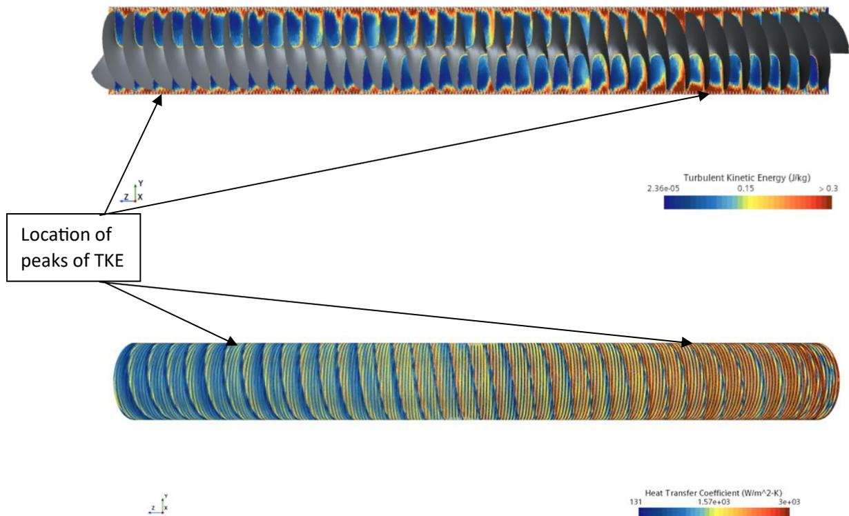
Figure 17 a. Scalar scene for the Turbulent Kinetic energy for tube 5035 b. Scalar scene for the Turbulent Kinetic energy for tube 5035
