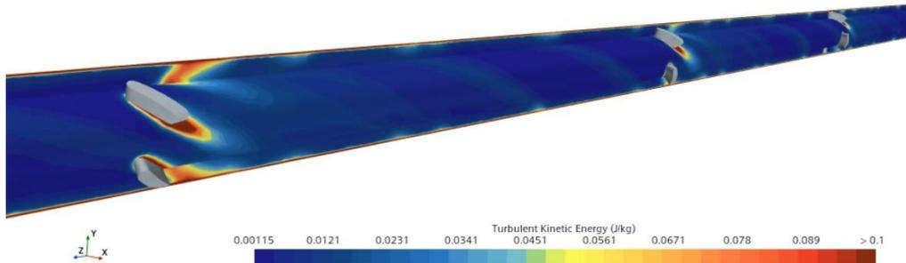
Figure 39 TKE for 12 cm spaced vanes at  $Re=42,000$
