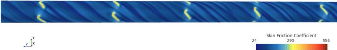
Figure 42 Skin friction coefficient for the 5cm geometry.
