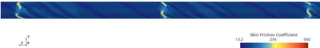
Figure 43 Skin friction coefficient for the 12 cm geometry.
