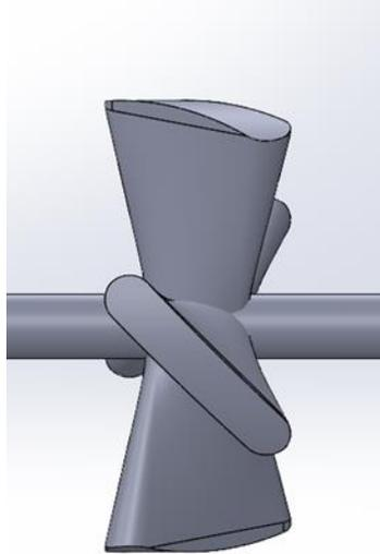
*Figure 20 Side view of the vanes.*
