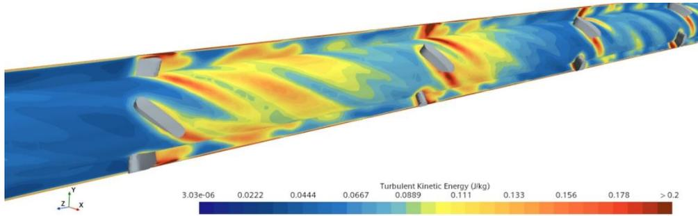
Figure 38 TKE for 5 cm spaced vanes at  $Re=42,000$
