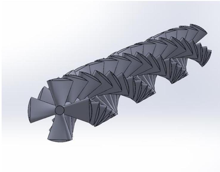
*Figure 19 Isometric view of the vane insert.*
