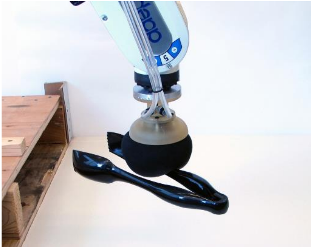
Figure 9: Grasping point strategy [16] for determining a rectangle for the ideal position for grasping an object. This refined other work as employing the “centroid method” since at every grasp, the gripper moved towards the centroid of the object.
