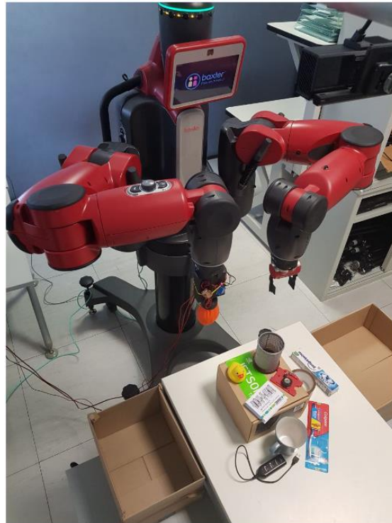
Figure 18: Baxter dual arm robot [32] which highlights the complementary role of GJG similar to [16] with GJG+EA. The GJG shown here may not be good for grasping the cup shown, where the parallel gripper would be. However, the duck and other small objects might be more difficult for a parallel gripper and simpler for the GJG.
