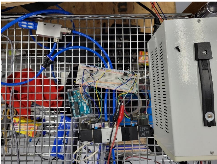
Figure 25: Physical system configuration for gripper control
