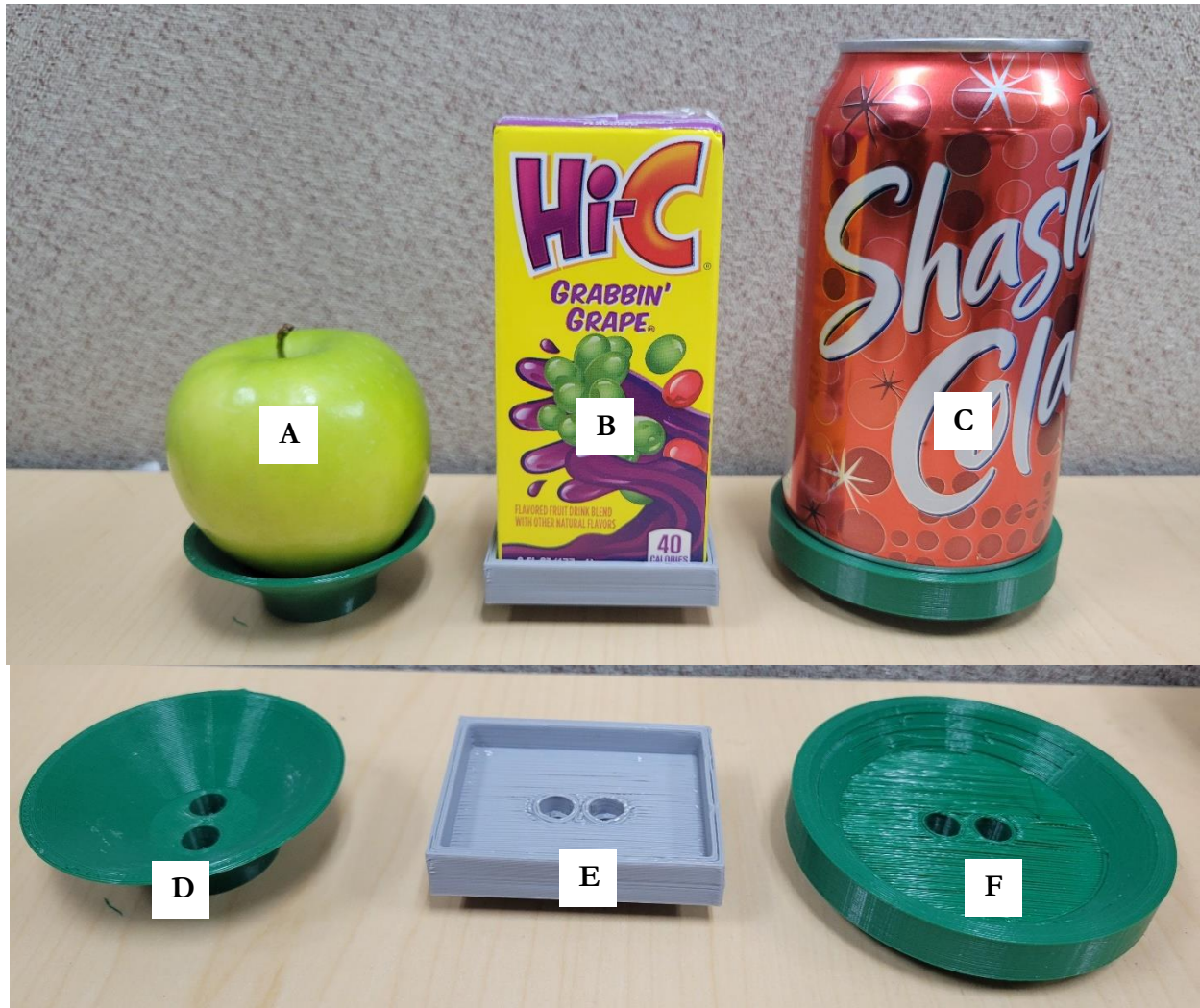
Figure 27: Picking objects for common object testing. A. Apple, B. Juicebox, C. Can; D, E, F: Load cell attachments for the three objects, A, B, C, respectively
