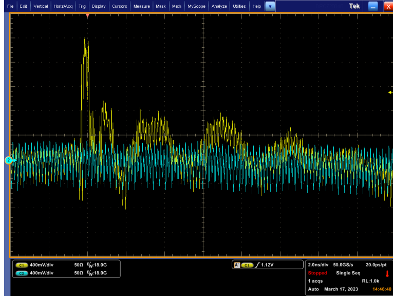
Fig. D.47 An oscilloscope capture is taken from the experimental setup demonstrated in Fig. D.44 where the linear antenna waveguide structure is placed external to an AWG 4 on a fixed axis translated at z = -10.2cm .
