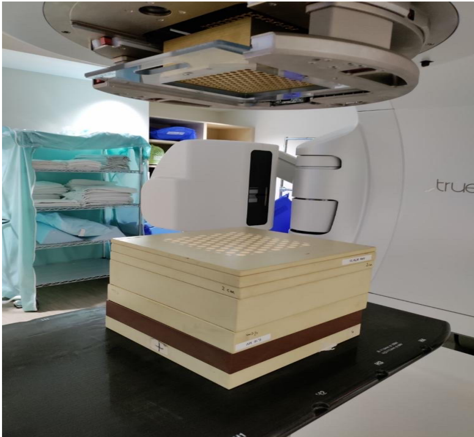
Figure 2: Set-up of the physical grid block for film measurements.
