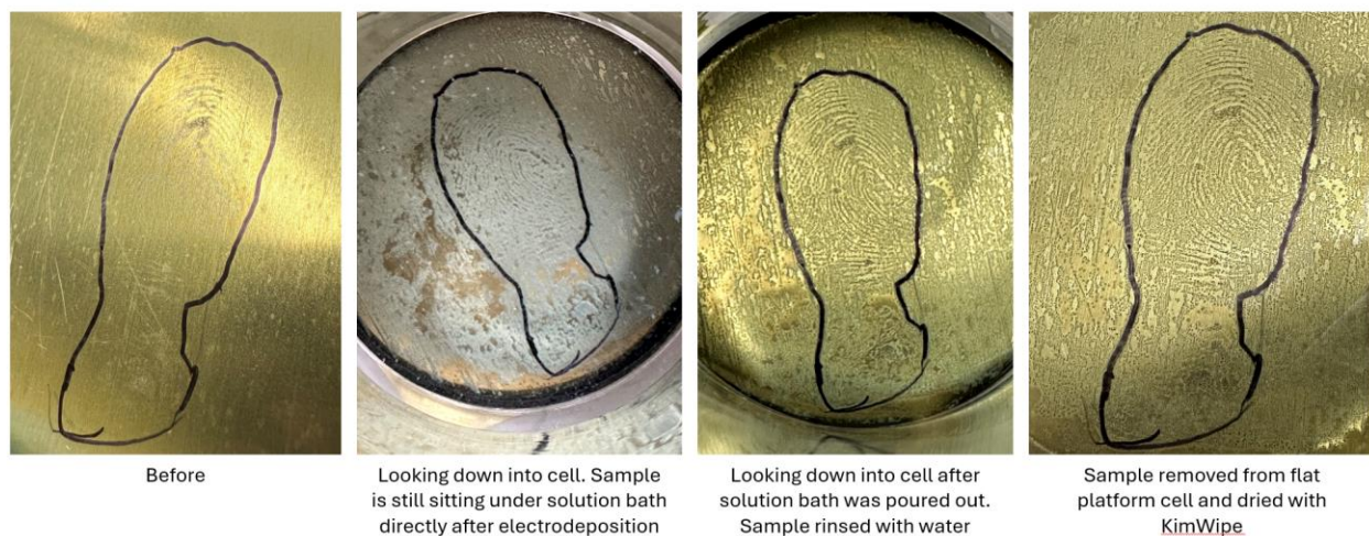
Figure 38: One of three trials of Au electrodeposited onto C260 brass using an applied potential of 4V for a total of 20 seconds. Images are taken before electrodeposition, after electrodeposition whilst still in solution, after electrodeposition solution has been poured off and the sample rinsed with ultrapure water, and lastly, after the sample has been removed from the flat platform cell and dried with a KimWipe
