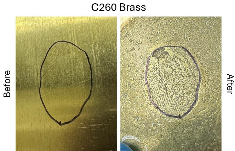
Figure 37: One of three trials of gold electrodeposited onto C260 brass using an applied potential of 4V for a total of 20 seconds
