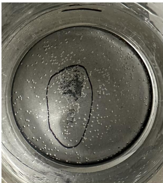
A. Sample held at 1V , image taken at 5 second mark when agglomerations began to form on substrate surface submerged in solution.
