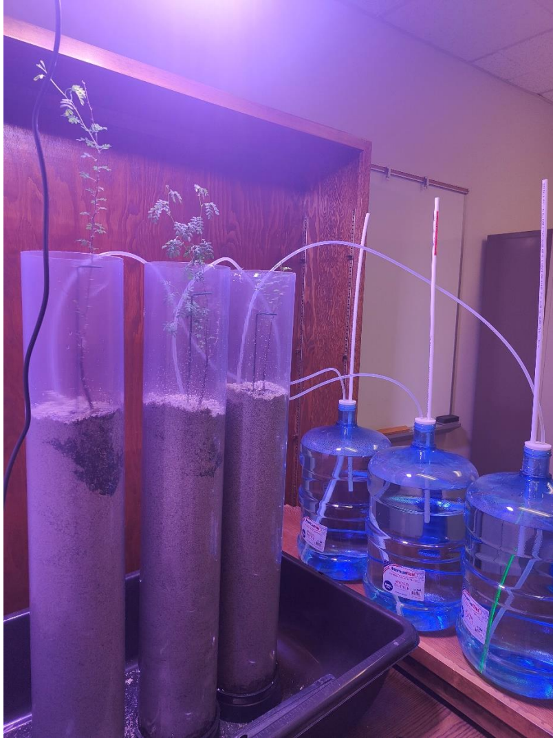
Figure S3.2. Experimental setup to study the root distribution of three screwbean mesquite seedlings under different groundwater level scenarios.
