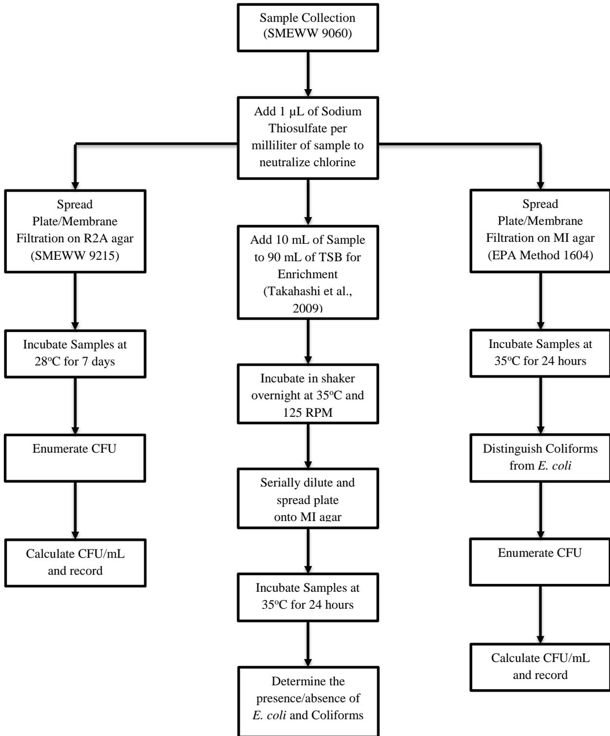
Figure 1. Flow Chart for ice and water sample collection and analysis on R2A and MI agar
